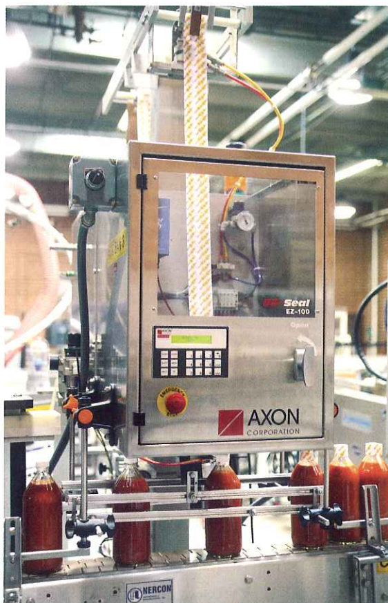
T-E BANDING. Tamper-evidencing bands are applied and heat-shrunk to the sauce bottles.
